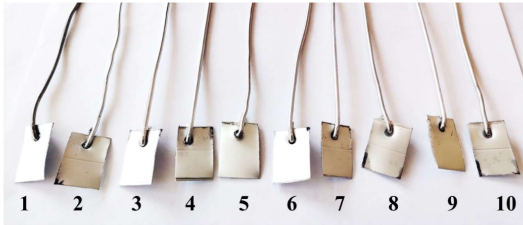
Figure 3. Samples after the anodizing process.
